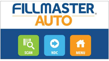
Touch "Scan" to turn on the scanner on the left side of the machine. Once activated, scan NDC on medication Touch "NDC" to type in the full 11 digit NDC Touch "Menu" to find more screens to help you learn more about the Fillmaster Auto
